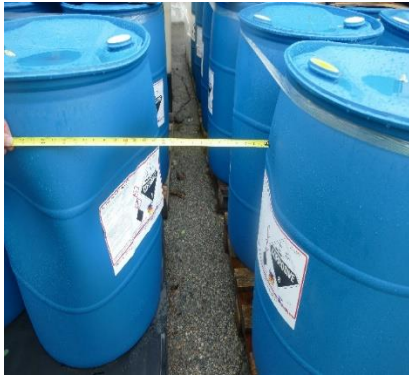
Insufficient aisle space between chemical drums.
