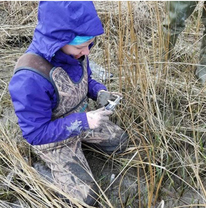
Measuring sediment accretion in a feldspar plot (WMAP)
