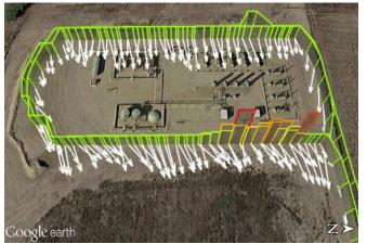
The adjacent figure provides an example of GMAP results from mobile monitoring for hydrocarbons. These results present the wind direction and speed that are used to identify the location of the emission source, as well as the relative concentration (represented from low to high by green to red) of the emissions at each geo-spatially identified location.
