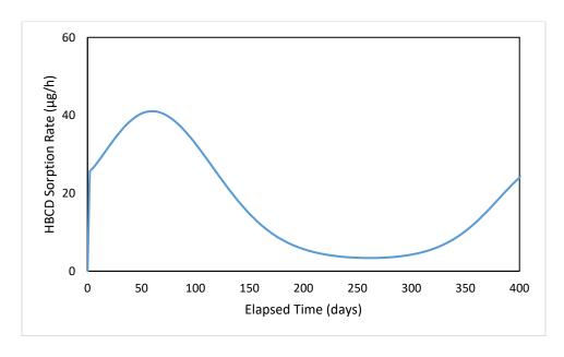
Figure Apx G-6. Rate of HBCD Sorption by Gypsum Board Walls
