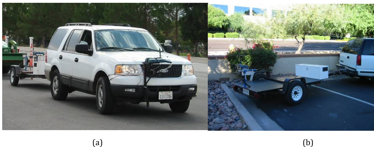
Figure 2. Example of PM sample inlet line that is located on a trailer behind the test vehicle. a. On the front end of the test vehicle, a sample inlet line is used to direct air to a nephelometer-style instrument that measures background PM; b. the sample inlet line located on the trailer behind the test vehicle is centered between the trailer tires. Both background and trailer sample inlet lines are equipped with an isokinetic sampling system.
