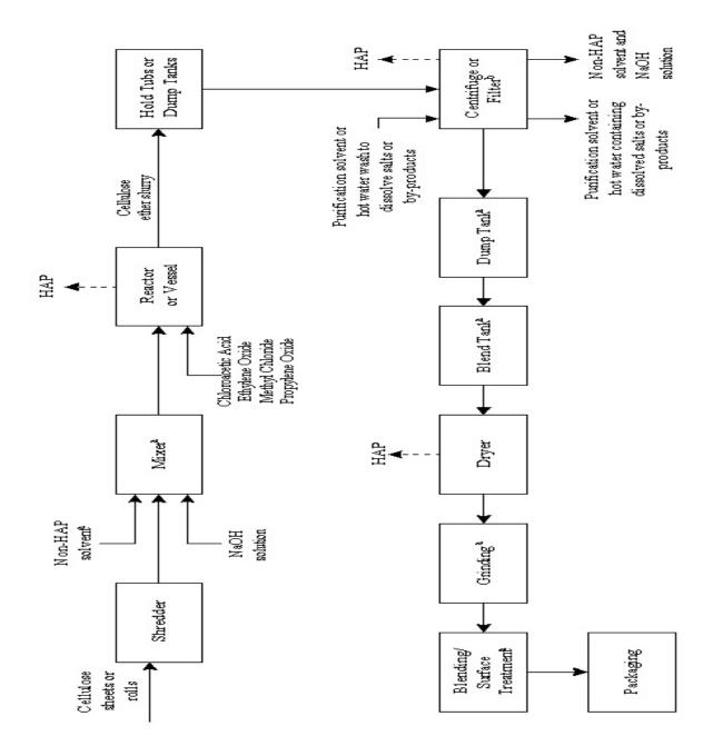
Figure 2-2. Cellulose Ether Manufacturing Process
