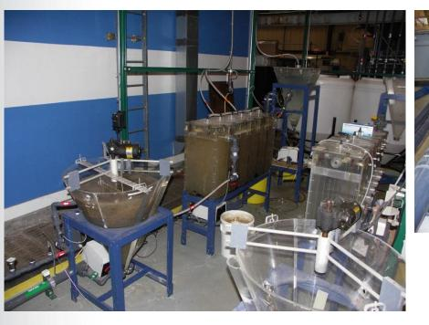
Activated sludge experimental set-up: assessing how contaminants travel through wastewater treatment systems Wastewater test bed: assessing persistence of contaminants on sewer infrastructure
