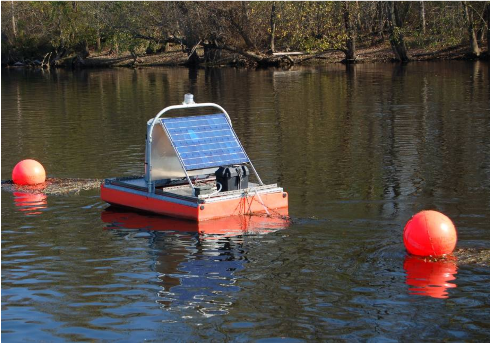
Figure 2-11. Floating monitoring station.
