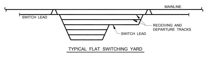
Figure 9-A-8 – Typical Flat Yard Arrangement
