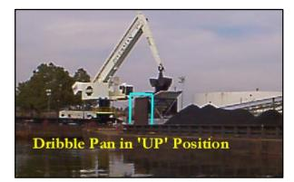
Figure 8-A-1 Unloader with Hopper and Dribble Pan
