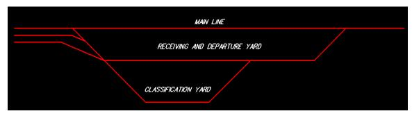
Figure 9-A-1 – Typical Flat Switching Yard
