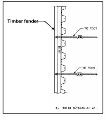
Figure 8-A-3 Timber Fendering
