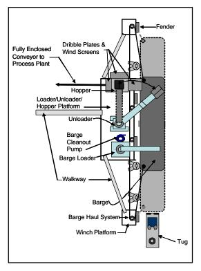
Figure 8-A-8 Pile-Supported Barge Berth
