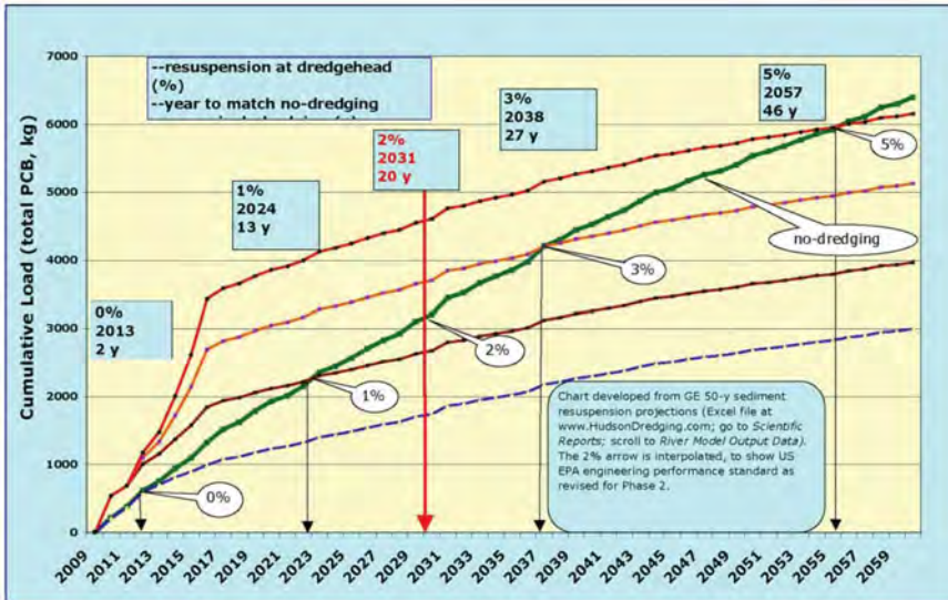
Figure 2. At Waterford: GE projected years needed to match no-dredging, assuming zero dredge mobilization of PCB other than ‘resuspension’.
