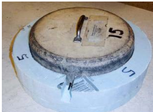
Large Area Activated Charcoal Canister (LAACC) Equipped with Float
