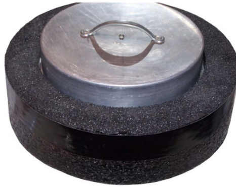
Method 115 Large Area Activated Charcoal Canister (LAACC) adapted to float on fluid surfaces (Homestake Mining of California)
