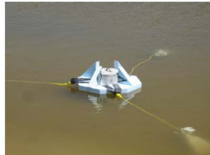
Styrofoam float with Large Area Activated Charcoal Canister (LAACC) Floating in Lagoon Tied to Anchors
