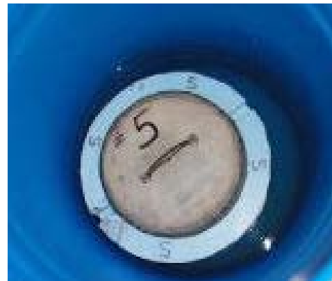
Large Area Activated Charcoal Canister (LAACC) Floating in Water Filled Barrel
