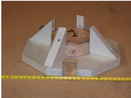
Styrofoam float with Large Area Activated Charcoal Canister (LAACC) on Floor
