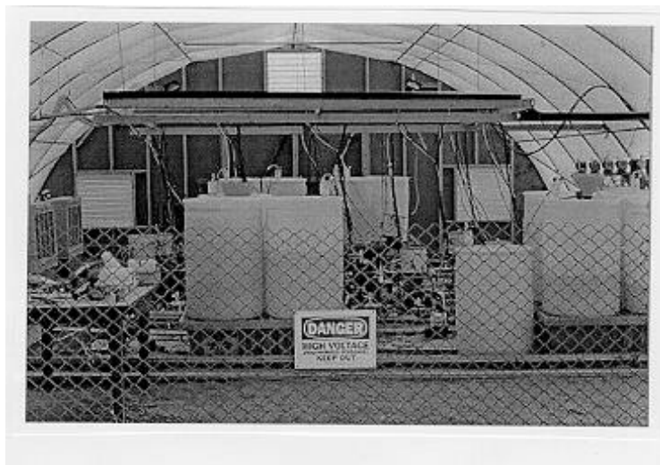
Figure 24 Electrokinetic demonstration for chromate removal at the Unlined Chromate Acid Pit (Sandia National Laboratories, Tech Area III, Chemical Waste Landfill) (Source: Sandia National Laboratory world wide web site at http://www.sandia.gov )
