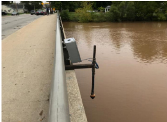
Figure 1. During heavy rainfall episodes, RTC technology monitors and notifies the city of rapidly changing water levels at the Mason Street Bridge.
