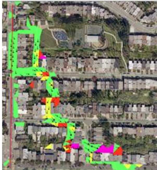
Figure 1. Overland flows transported on the ground surface, as shown in the two-dimensional module.
