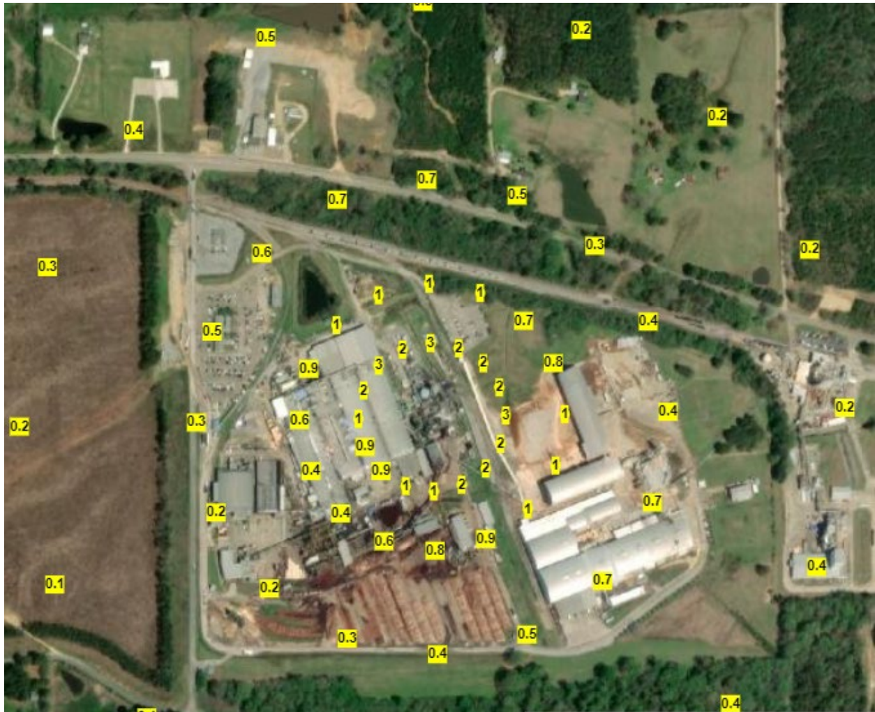
Figure 11. Aerial photo of Facility 7984011 and corresponding acute RELs for formaldehyde at HEM-4 polar receptor locations.
