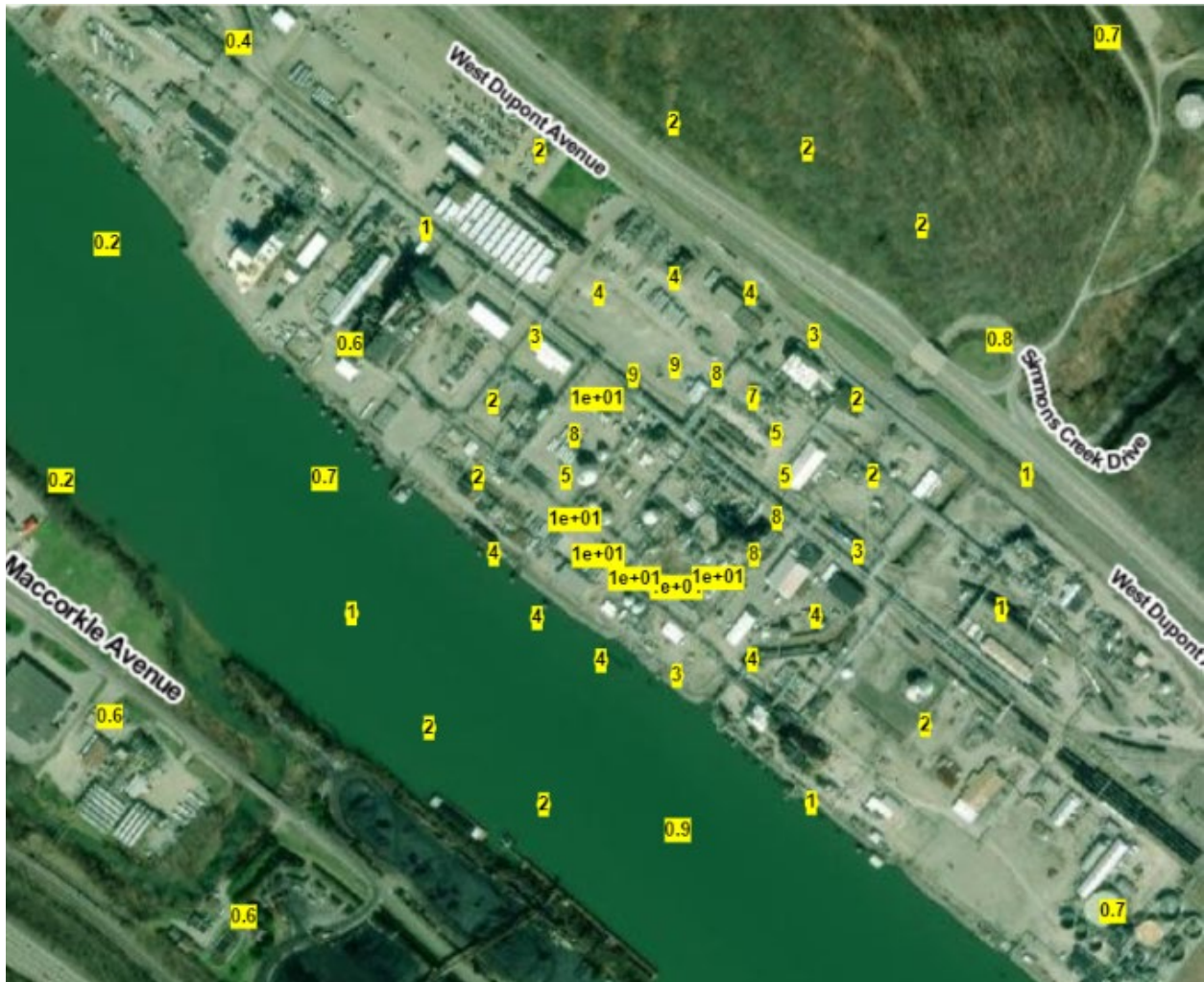
Figure 1. Aerial photo of Facility 6884211 and corresponding acute RELs for formaldehyde at HEM-4 polar receptor locations.
