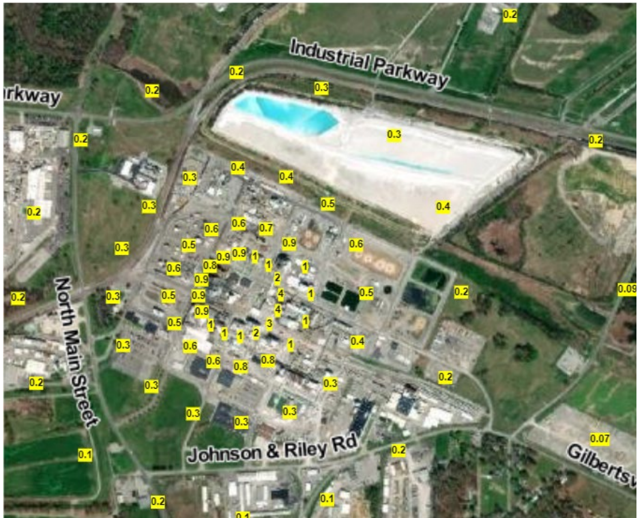
Figure 7. Aerial photo of Facility 8096711 and corresponding acute RELs for methanol at HEM-4 polar receptor locations.
