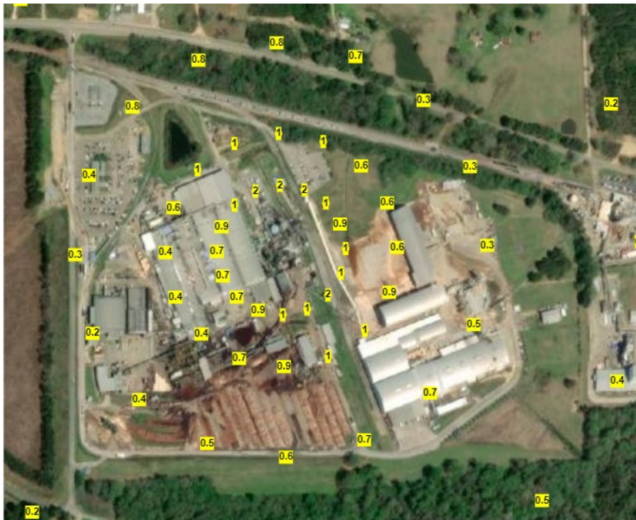
Figure 16. Aerial photo of Facility 7984011 and corresponding acute RELs for acrolein at HEM-4 polar receptor locations.
