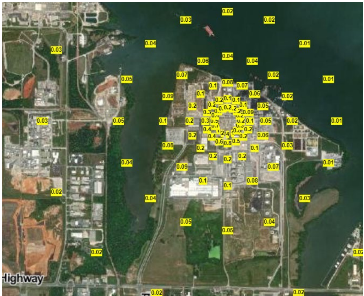
Figure 21. Aerial photo of Facility 985511 and corresponding acute AEGL2s for acrylonitrile at HEM-4 polar receptor locations.
