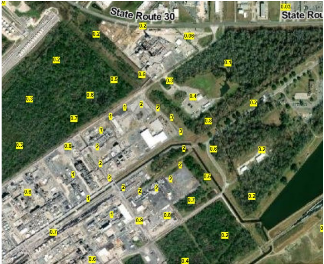
Figure 10. Aerial photo of Facility 7367211 and corresponding acute RELs for methylene diphenyl diisocyanate at HEM-4 polar receptor locations.
